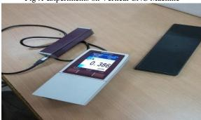
Fig.2 Mitutoyo Surftest SJ-201P Instrument
